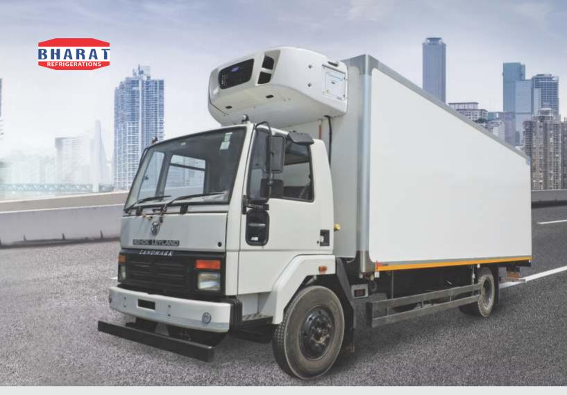
Bharat Refrigerations Refrigerated container is designed to transport with options of different temperature range (+15°C to -25°C) for all perishable foods on all type of vehicle such as small, mini truck & heavy loading truck.
